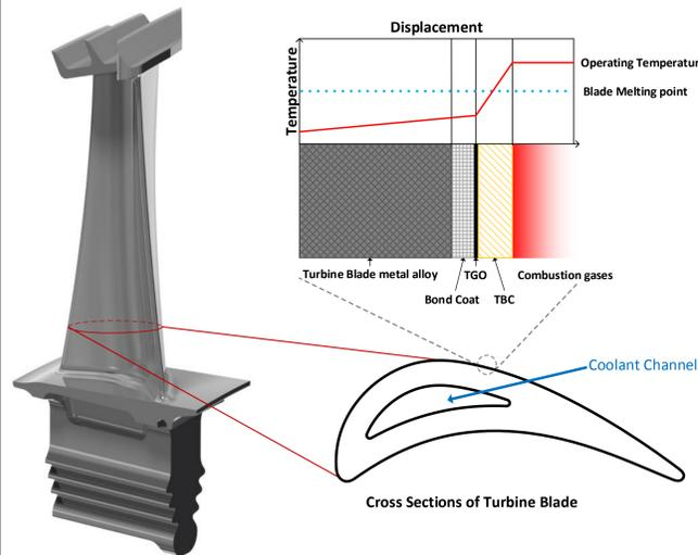
The thermal barrier coating (TBC) is adhered to the surface of the turbine blade by a nickel based bond coat and the blade is forced cooled with air by an internal coolant channel.
