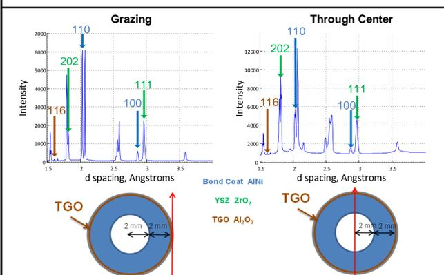
The Bond Coat, TGO, and YSZ were identified in both the scans through the center of the sample as well as the scans near the surface. Noise is more prevalent in through-center scan due to the diffracted X-ray beam passing through the material more than once.
