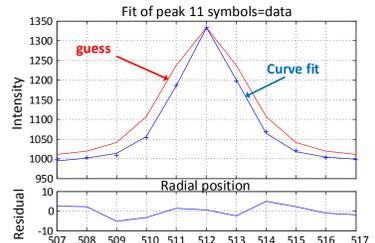
The radial position around the azimuthal angle is then measured for each experiment. With this, the strain is then calculated based on the radial displacement around the azimuth.
