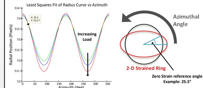
The mechanical loading is varied to determine the zero strain reference angle. This zero strain angle is independent of temperature.
