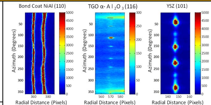
The diffracted rings were integrated azimuthally to create a radial plot. Shown are the Bond Coat, TGO and YSZ Rings. The double bell curve shown in these lines indicates that strain is being experienced by the material.
