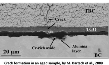
The aged samples will have a more developed and thicker TGO layer due to added cycles.
