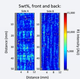
It can be seen the in the 5wt% sample (above), the particles are well dispersed. On the other hand, particulate sedimentation can be observed in the 20wt% sample (below).
