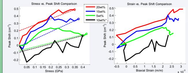
Digital image correlation was conducted simultaneously, and complimented the non-contact piezospectroscopic sensing. Strain data showed similar trends to those observed with photo-luminescent mapping. It also appears that if the particles do not reach the de-bond point, they unload to a positive peak shift. On the other hand, if they de-bond, they unload to a negative peak shift.
