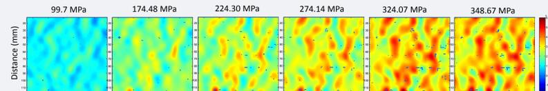
The average peak shift of each map at its respective stress and strain are plotted to the right, and a linear ramp-up behavior can be observed in both, the slope of which quantifies the PS coefficient (stress sensitivity). The PS error bars are representative of the non-uniformity of the surface, and the DIC strain data also reflects this surface non-uniformity.
