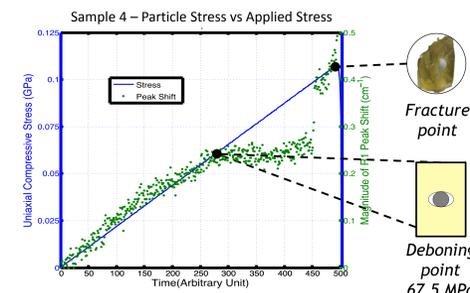
All isolated particle results follow the trend above in which the particle sustains load up to a certain point, and then maintains a constant peak position. This could be due to the particle deboning from the matrix.
