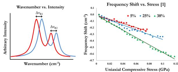
Our previous work showed that by embedding alumina nanoparticles within an epoxy matrix, the piezospectroscopic sensitivity to applied stress on the nanocomposite could be tuned with respect to particle volume fraction [1].
