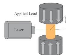
The experimental set up contains a load frame which places the sample in compression, while PL data is collected by utilizing a laser excitation source.
