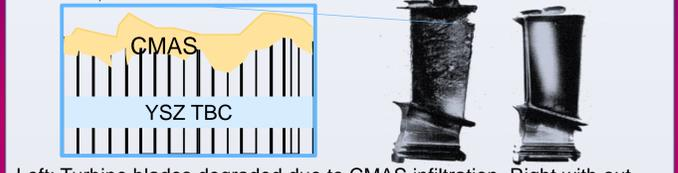
Left: Turbine blades degraded due to CMAS infiltration. Right with out CMAS.
