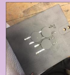
Samples after grit-blasting attached to a mounting plate
