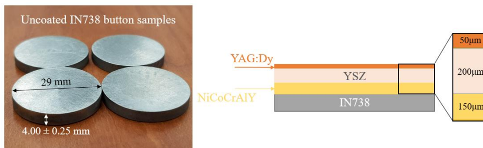
Figure 3: Dimension of the uncoated IN738 button samples and thickness of the coating of the calibration samples
